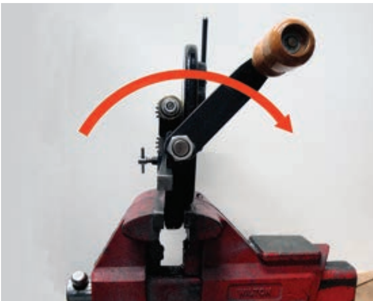
(Figure 2) Proper hand crank rotation as viewed from side.
