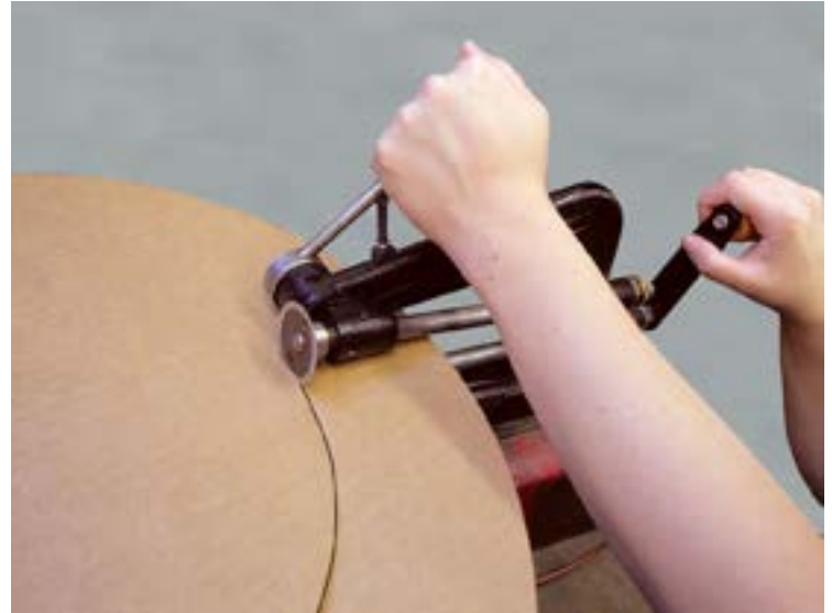
(Figure 8) To cut the inner diameter (ID), loosen the scale bar T-screw, and slide the scale bar to the desired setting. Hand tighten the scale bar T-screw. Engage the top cutting disc. Turn the hand crank, simultaneously maintaining downwards pressure on the cutting disc lever as before. Continue cranking until the entire ID of the gasket material has been cut. Disengage the top cutting disc and remove newly cut gasket. Unscrew and remove knurled nut from spindle. Discard unwanted material.
