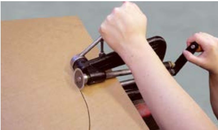
(Figure 7) Turn the hand crank clockwise. Simultaneously, with the other hand, maintain a constant downward pressure on the cutting disc lever. As the cutting discs rotate, the gasket material will be drawn towards the cutting discs initiating the cutting process. Continue cranking until the entire OD of the gasket material has been cut. Disengage the top cutting disc. Discard unwanted material.
